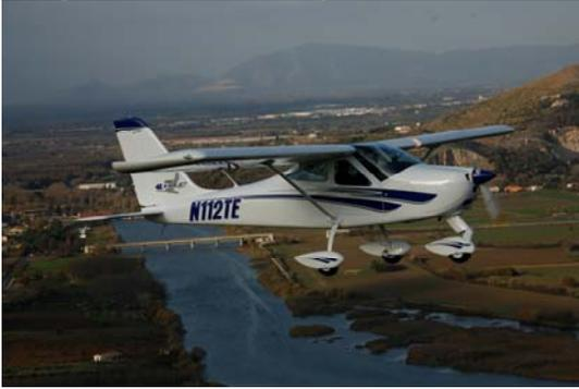
The Tecnam P92 Eaglet is a high-wing light sport aircraft, with a useful load of 540 lbs. Its Rotax engine burns approximately 5.3 gph while cruising at 116 knots, giving the Eaglet a range of over 500 miles.
